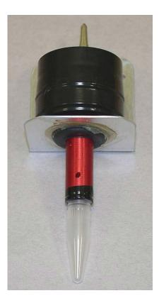
Assembled single-stage BC 112 sampler: The tubes and filter cassette on the BC 221 are sealed with tape as shown. Note that the sampler inlet must face forward.
