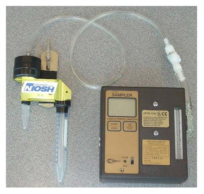
**Two-stage BC 251 sampler attached to personal sampling pump:** Note that the white CPC quick-disconnect fittings contain valves that shut off the fitting when they are disconnected. Because of this, do not turn on the pump while the sampler is not connected; the pump will not be able to draw air and will shut down.
