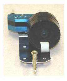
Top view of BC 221: To mount the sampler on the holder, slide the nylon retainer onto the filter cassette and press the sections of Dual Lock strip together. Pull them apart to remove the sampler.
