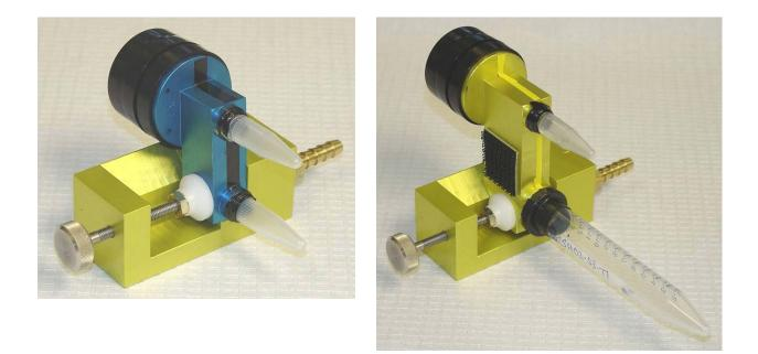
The calibration adaptor is shown here with a BC 221 sampler (left) and a BC 251 sampler (right) properly inserted.
