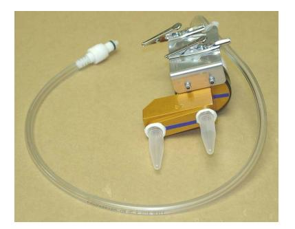
Rear view of BC 212 sampler: The stainless-steel L-bracket allows the sampler to be clipped onto a worker. This bracket attaches with two socket-head screws as seen. The bracket can be removed if it is not needed. The bracket has four holes for alligator clips (two clips are shown). The clips can be rotated or moved to different holes as desired.
