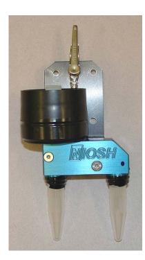
BC 221 sampler: The tubes and filter cassette on the BC 221 are sealed with tape as shown rather than caulk. The seam around the sampler is sealed with tape to prevent air leakage during conductive polypropylene.
