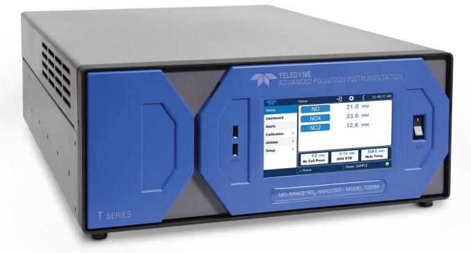
The Model T200M Mid-Range NO / NO<sub>2</sub> /NO<sub>x</sub> analyzer uses the proven chemiluminescence detection principle and advanced electronics to allow accurate, dependable, continuous measurements for mid-level stack gas monitoring and other applications. The T200M may be fitted with an optional, internal paramagnetic O<sub>2</sub> sensor or an infrared absorption CO<sub>2</sub> sensor, reducing integration and operating costs significantly.
